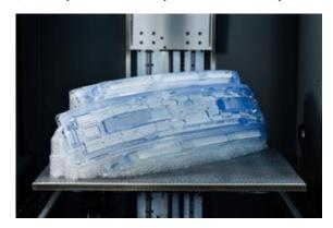
Covestro's additive manufacturing business includes one of the world's most recognized and trusted brands in photopolymers - Somos. The automotive grill shown here on a Stratasys Neo800 stereolithography system was 3D-printed with clear Somos WaterShed CX 11122.
